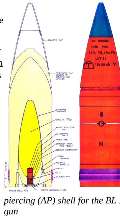
Figure 6: Armor piercing (AP) shell for the BL 15-inch Mk I naval gun
